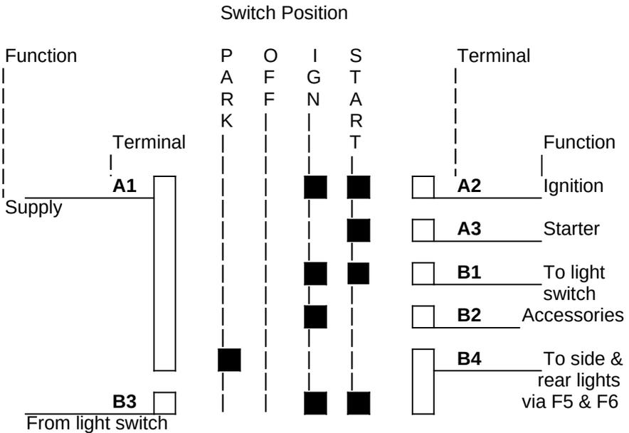
When reading this diagram, the connections are to the open rectangles, or squares at the sides, There is a connection across the diagram where a black square is shown in the selected position. For example in the PARK position, the supply at A1, is connected to the side & rearlights at B4,. There are no other connections with the key in this position.
