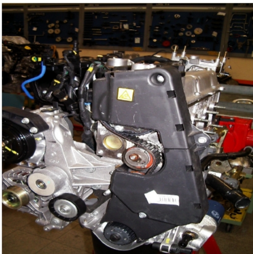
Protection of the upper and lower timing belt
