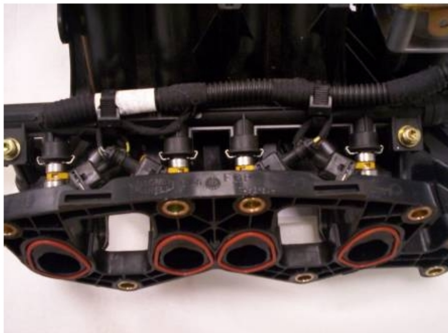
Housing injectors on the intake pipe
