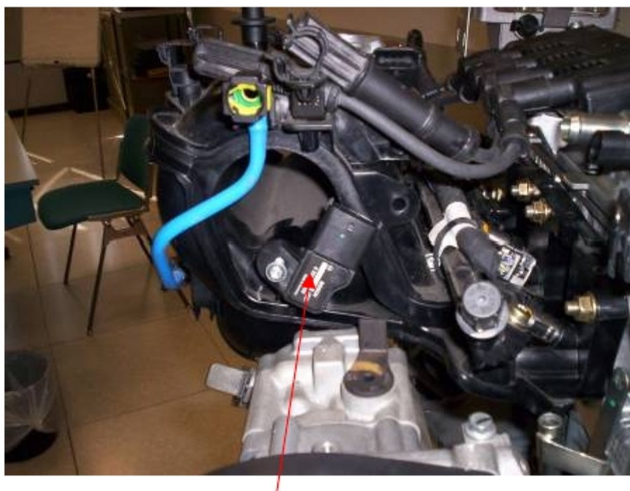
Temperature sensor / Intake air pressure
