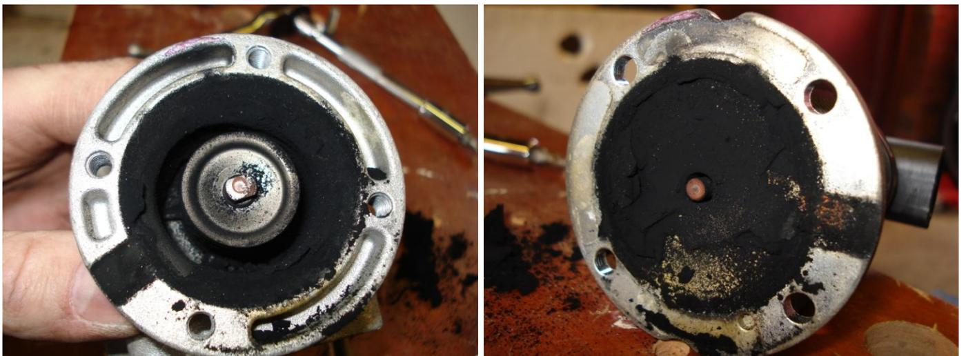
This is all the soot and muck that fell out, and scraped out between the EGR solenoid and EGR body !
