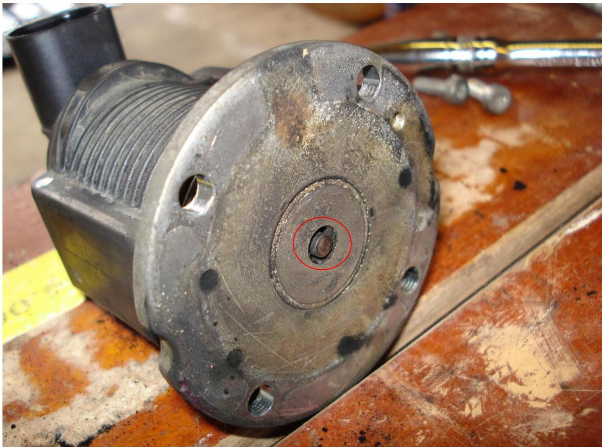
Securely hold the EGR solenoid in a vice or work bench. Drill a hole 3mm to 4mm in diameter in the plastic as shown in the picture. Next take a 3mm or 4mm punch to the inside of the solenoid, and knock out the insides. It might take quite a bit of force... be brave... and catch the insides when they come out !
