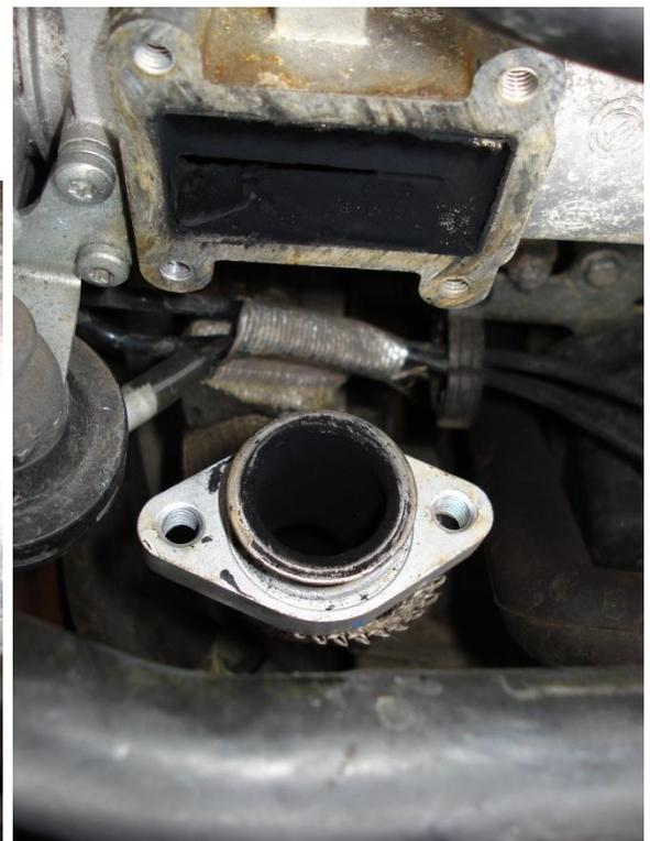
Next step is to remove the EGR solenoid from the EGR valve body, it's held on with 4 x T25 Torx bolts.
