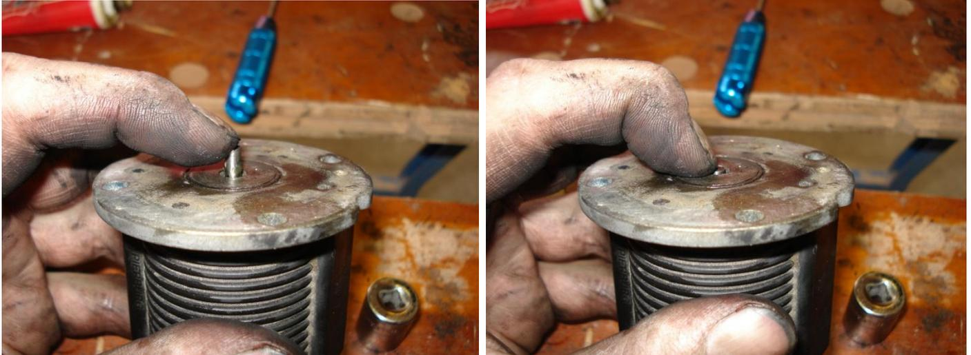
Dry out the EGR body that has been soaking in Carb Cleaner, and re-attached to the Solenoid. Remember the mark you made earlier? Align the marks.
