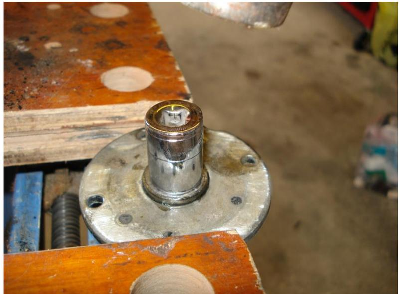
Once it's all back in place, the pin on the solenoids internals should easily be able to move in and out, it should be sprung to the out position. If you can't push it in and out with minimal effort, a little more cleaning may be required.
