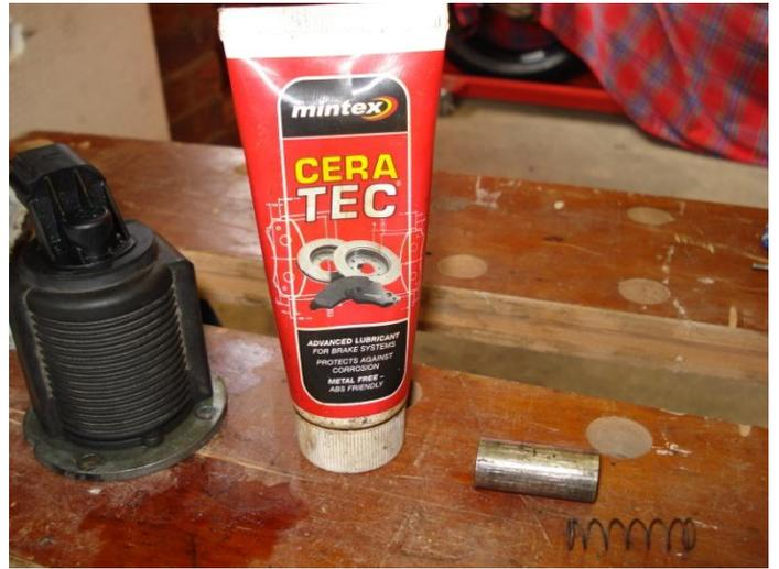
Fit all parts of the internals back together, and slide the solenoid body back over them. Turn the solenoid back over and hold again the vice or work bench, and using a socket knock down the end of the internals so they are flush with the housing.
