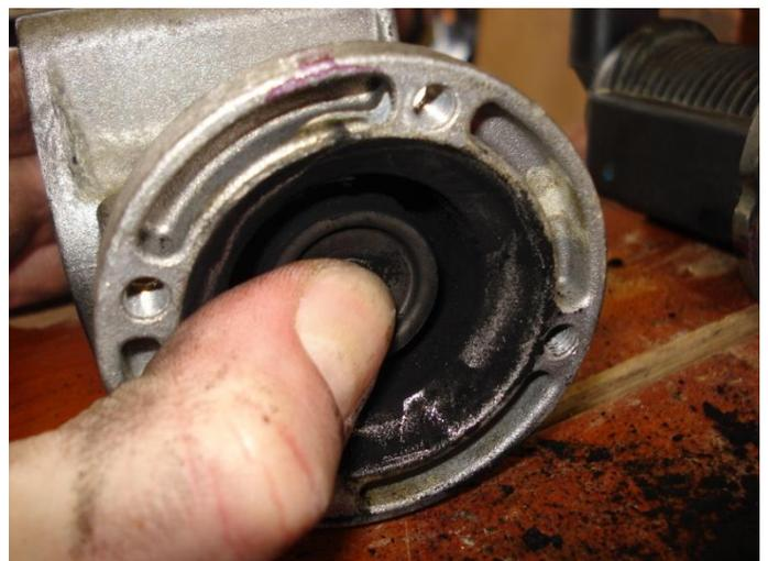
Next, find a suitable tub to put the EGR body into while it has a little bath. Give it a good dose of Carb cleaner, the Carb Cleaner comes out at quiet a pace, so it's idea for blasting away loose soot and dirt. (Don't go squirting yourself in the eye, like me ☺)
