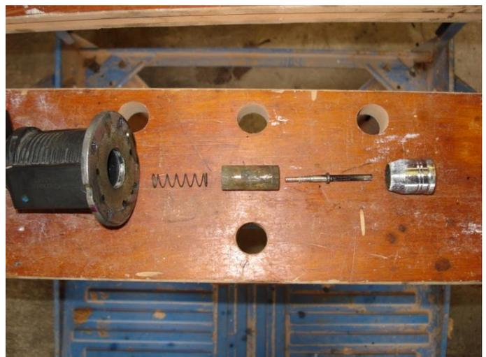
Clean up all parts of the solenoid, with a little wet 'n' dry paper or similar. Clean out the inside of the solenoid casing. Smear the solenoid with grease, I used Ceratec, but I'm sure it doesn't make a huge difference, although I'd shy away from copper slip, it obviously not ferrous, so will not be affected by the electromagnet but, all the same..
