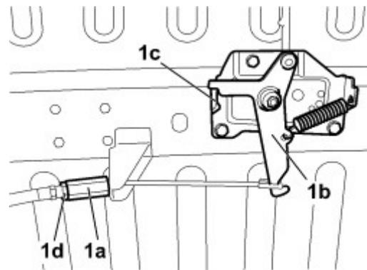
1. With the handbrake lever in the rest position, work underneath the vehicle and tighten the adjustment nut (1a) until the lever (1b) slowly becomes detached from the end of travel position on the bracket (1c); then lock the locknut (1d).
