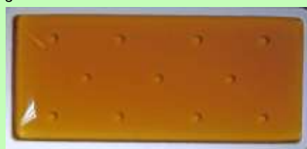
Control slide taken from clean fuel sample and incubated alongside the slides above. No contamination found.
