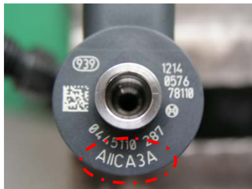
Bosch injector generation 2 IMA code for injector flow adjustment
