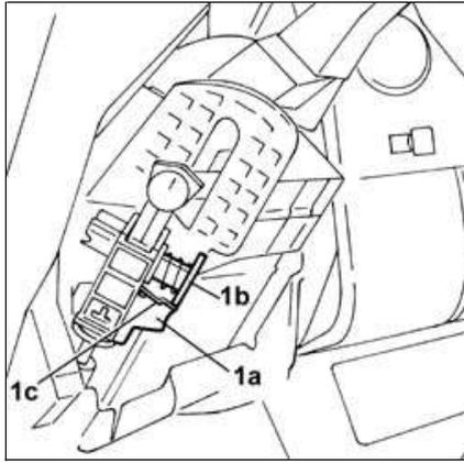
1. Lower the lever (1a) and push the button (1b) forwards as far as the splining (1c).
