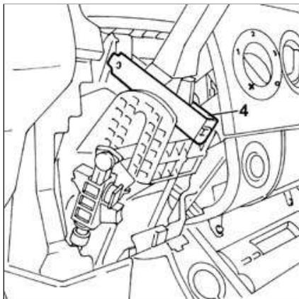
1. Position a 1.2 mm shim between the gear lever and the barrier.
