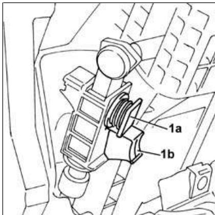
1. Release the lever (1a) so as to lock the button (1b).
